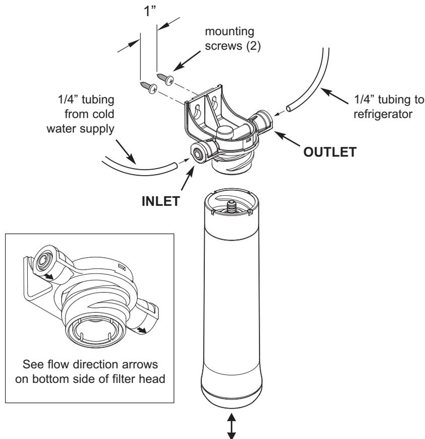
**NOTE:** Be sure to allow a minimum space of 1-1/2" under the system for removing the filter cartridge to change it.
