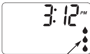
Droplets indicate water flow through conditioner
