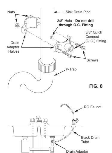
**IMPORTANT:** Do not install drain adaptor below the P-Trap. Locate drain adaptor so that when the black drain tube from the Reverse Osmosis Faucet is installed it will run straight to the adaptor, with no dips, loops, or kinks.
